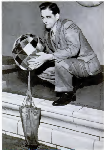
Reflecting marker buoy with its canvas sea anchor
